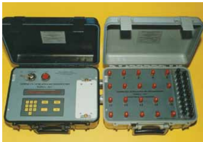
Rys. 3. Zapalarka milisekundowa EXPLO-201 [3] Fig. 3. EXPLO-201 millisecond exploder [3]
